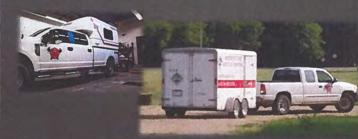
D1,D3,N14,N16,N17,N18 6 Air Trailers Full Air Cascade System Able to fill Self Contained Breathing Apparatus (SCBA) on location
